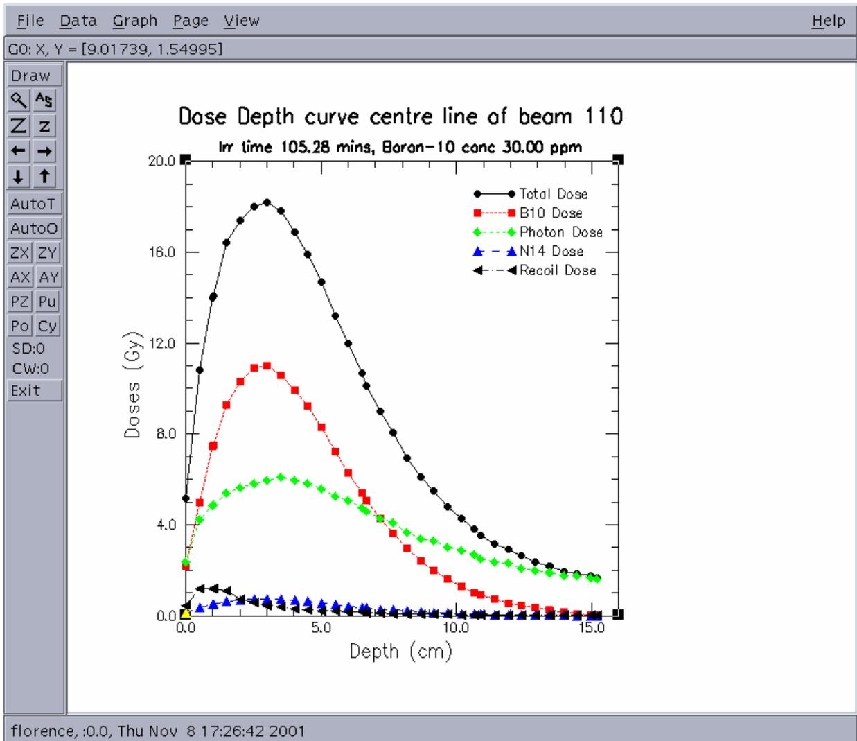
Figure1. Depth dose curves of the different dose component along the beam axis
