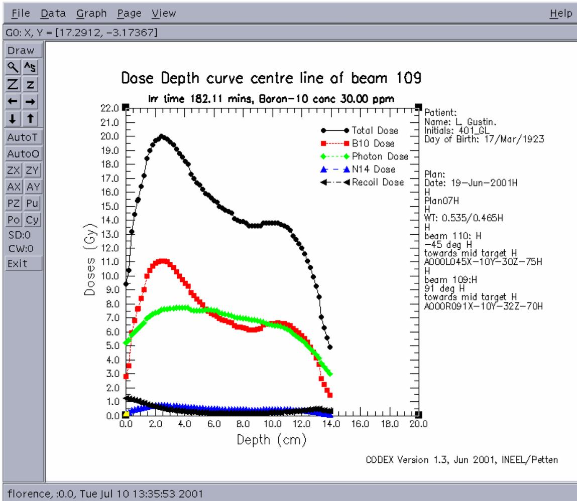
Figure 3. Doses depth curves of a 2 fields plan along the first beam axis
