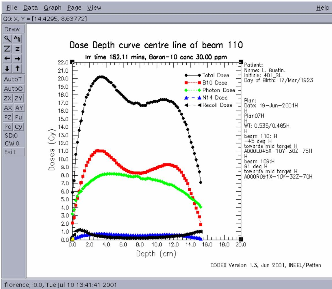
Figure 4. Doses depth curves of a 2 fields plan along the second beam axis
