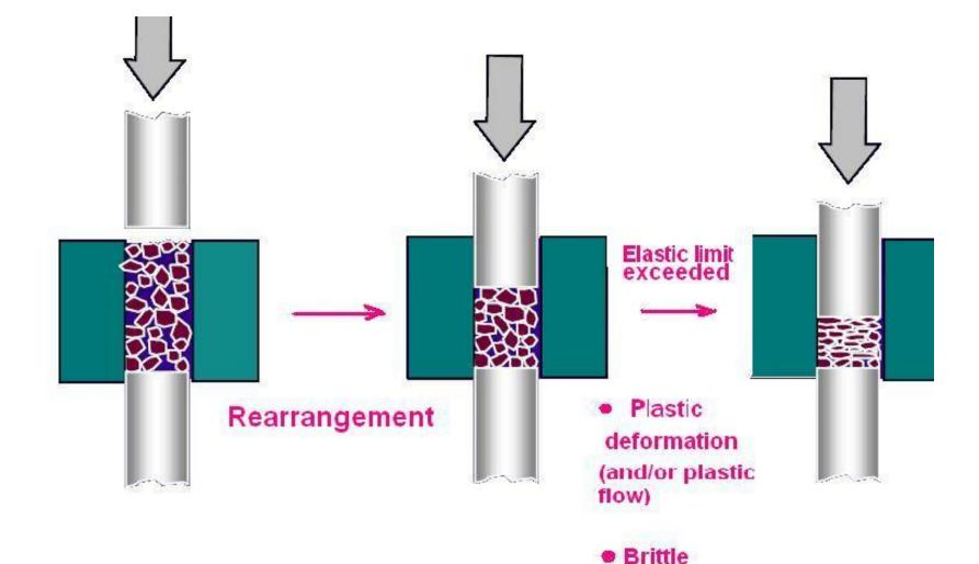
Plastic materials: when materials are ductilethey deform by changing shape(plastic flow).They are two elemetary processes:
