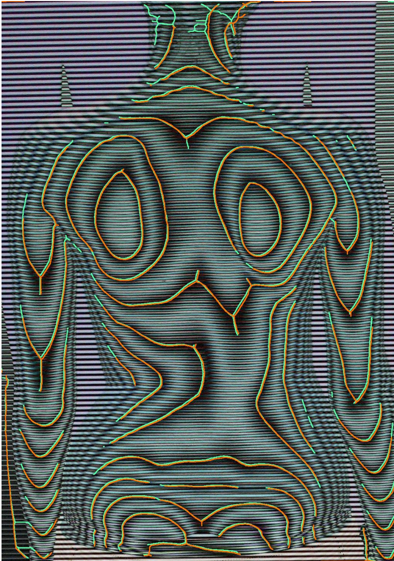
Fig. 17: Static (orange) and adaptive (green) segmented moiré fringes on image no. 3—displayed merged.
