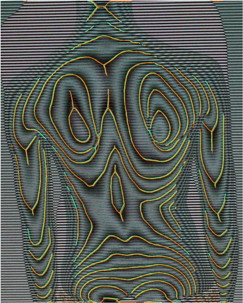
Fig. 15: Static (orange) and adaptive (green) segmented moiré fringes on image no. 2—displayed merged.
