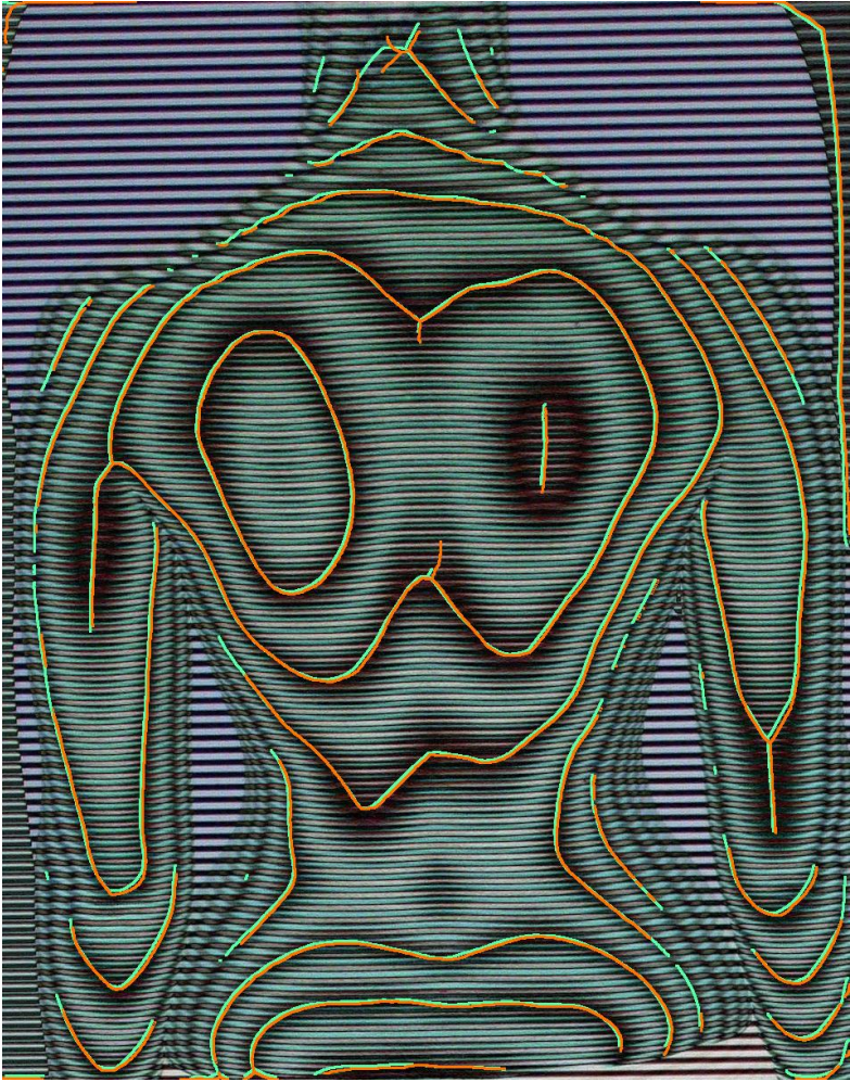
Fig. 13: Static (orange) and adaptive (green) segmented moiré fringes on image no. 1—displayed merged.
