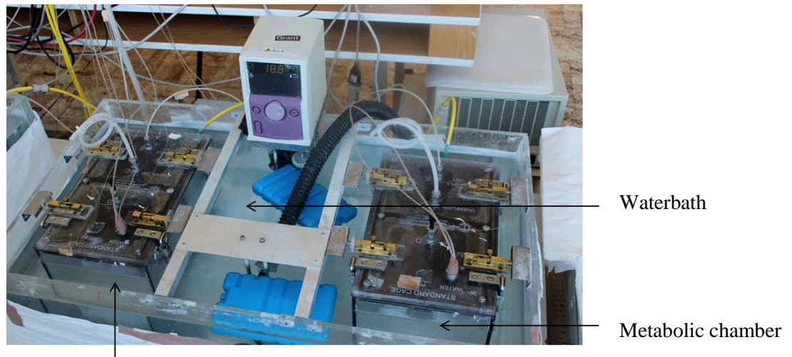
Figure 5. Oxymax indirect calorimeter system with metabolic chambers complemented with thermocouples and Benchtop thermometer for measuring thermoregulatory and metabolic functions.
