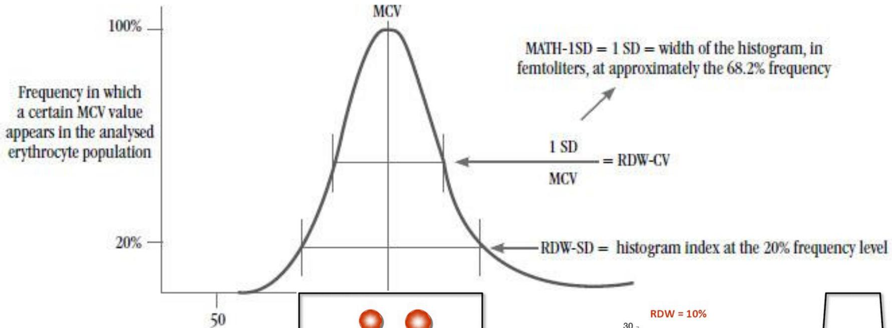
**FIGURE** – *Obtainment of RDW-CV, MATH-1SD and RDW-SD*
